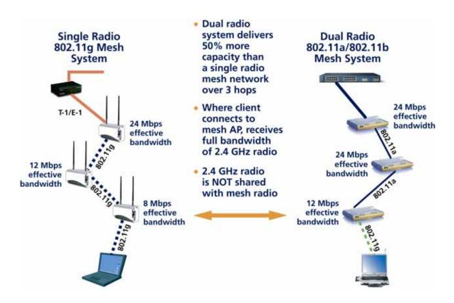
With the Proxim solution, the 5 GHz radio can be dedicated to the mesh network, leaving client traffic to the 2.4 GHz radio. This means that a standard three-channel 802.11b or 802.11b/g network can be built out maximizing system performance.
