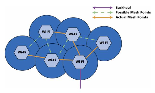
As additional Wi-Fi cells are added to increase coverage or capacity, Proxim's OMCP will automatically recalculate all paths and update routes as necessary, and connect in the new devices. Automatic network organization ensures that time-consuming field configuration is not necessary. APs are simply plugged in, and within minutes are operating as part of the network.
