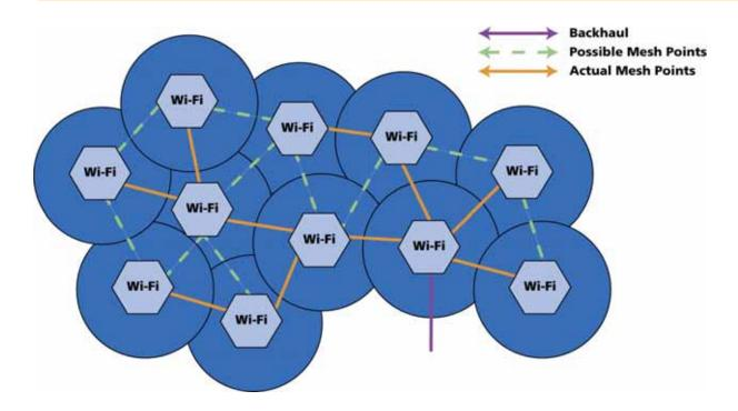
The ORiNOCO Mesh Creation Protocol is always dynamically calculating path efficiency for all possible routes. Each mesh AP secures a connection to all possible adjacent mesh APs. However, only one link is allowed to be open. Securing each possible connection in advance allows almost instantaneous path updates. The dynamic nature of OMCP is continuously checking for changes in the topology and environment. Changes in the network such as —
