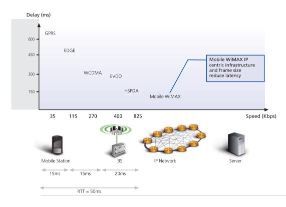
Figure 7: Comparing Latency WiMAX vs. The Competition (ms) Source: Intel [4]
