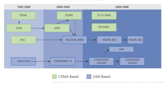
Figure 5: Cellular Network Evolution Source: Intel [2]
