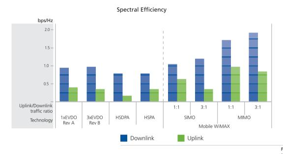
Figure 9: Mobile WiMAX Vs. 3G spectral efficiency comparison Source: WiMAX Forum [10]
