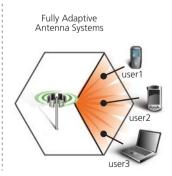
Figure 4: Beam Forming
