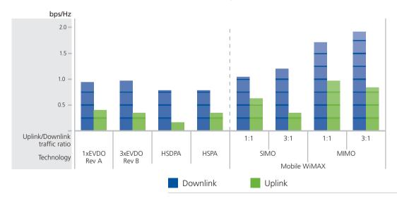
Figure 2: Performance comparison between WiMAX and 3G technologies: spectral efficiency Source: WiMAX Forum [10]
