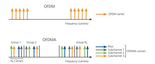
**Figure 3:** Single-carrier and OFDMA received signals
