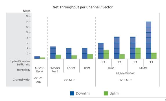
**Figure 1:** Comparison of WiMAX Vs. leading 3G technologies: net throughput per channel / sector
