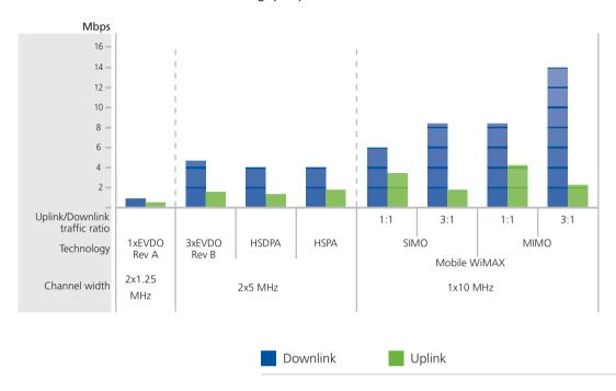
Figure 10: Mobile WiMAX Vs. 3G Net Throughput Comparison Source: WiMAX Forum [9]
