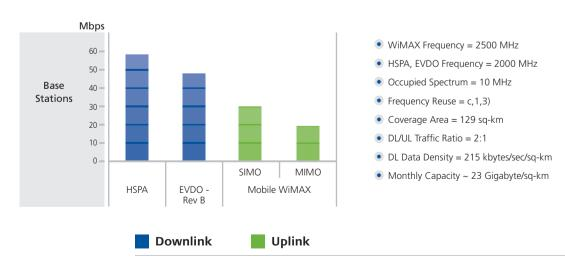
Figure 11: Mobile WiMAX Vs. 3G Number of required sites Source: WiMAX Forum [16]
