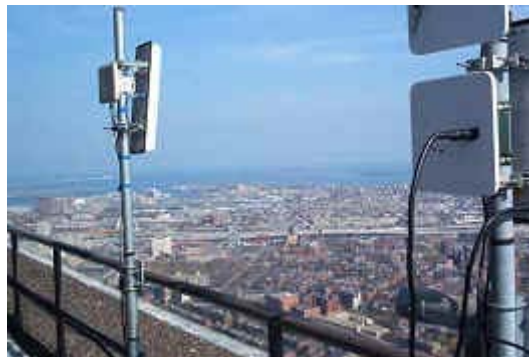
Example of an 802.16-style base station on the Prudential* Tower in Boston.
