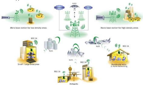
Typical point to multipoint Broadband Wireless Access (BWA) systems are composed of two key elements: base station and subscriber equipment. The base station connects to the network backbone and uses an outdoor antenna to send and receive high-speed data and voice to subscriber equipment, thereby eliminating the need for extensive and expensive wireline infrastructure and providing highly flexible and cost-effective last-mile solutions.
