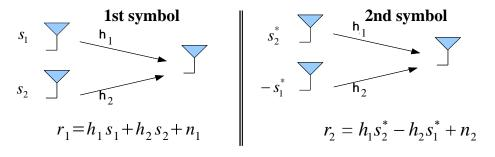
The receiver can apply proper decoding so as to retrieve the originally sent signals:
