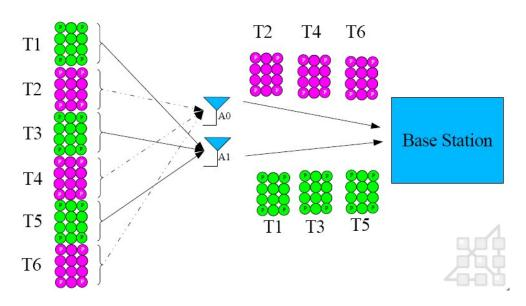
Because coding is performed on a slot-by-slot basis, the diversity introduced by TSD on the tiles will be exploited by the convolutional encoder to reduce the error probability. The exact order of diversity is directly a function of the coding order. Furthermore, a TSD scheme can be further enhanced by the use of MRC at the base station.
