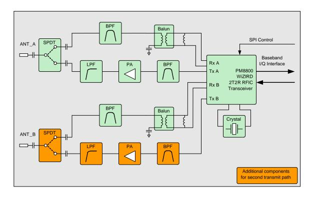
The additional size required for the additional components is approximately 50 mm<sup>2</sup> (this will vary depending on the components chosen). In the future, this could even be smaller, as integrated front-end modules (FEM) are used. Note that some FEM vendors are planning integrated dual-FEM designs in a single package. This process would further reduce the impact of the second transmitter.
