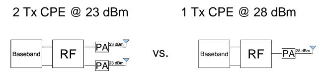
Considering that the dual-transmit terminal is implementing TSD, both terminals have equivalent performance in terms of link budget.
