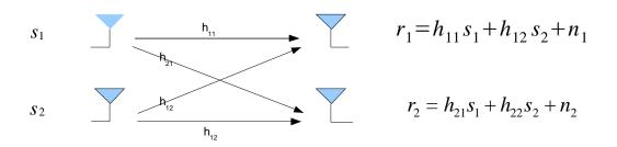
Decoding the stream of transmitted symbols requires that the channels be sufficiently de-correlated. Several decoder options are available, and the best performance is achieved with a maximum likelihood (ML) decoder. Sequans has implemented a maximum likelihood decoder as part of its patent-pending *mimo*MAX<sup>TM</sup> technology. Further explanation can be found in [3]. Note that this scheme requires 2 Rx antennas.
